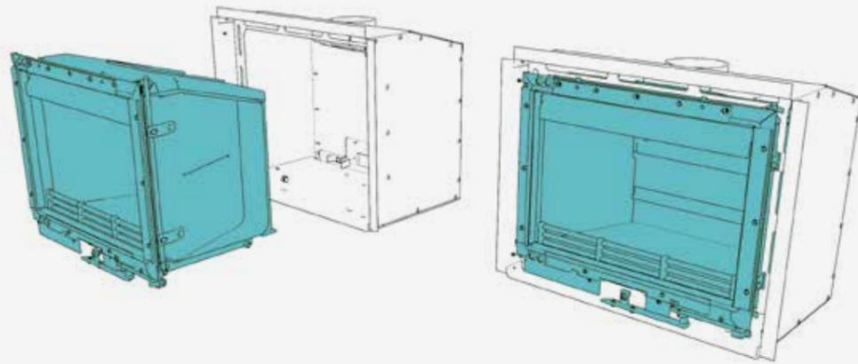
For easier installation of the R5 and R6 we have developed a convection chamber that can be fitted as a separate unit from the firebox.
